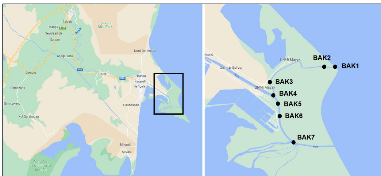
Figure 9: Map of measuring points for saltwater intrusion into the Kura River delta in October 2022h
